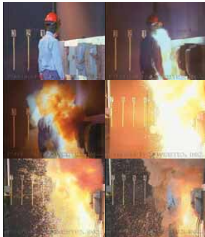
NFPA 70E states, "employees shall wear FR clothing wherever there is a possible exposure to an electric arc flash."
