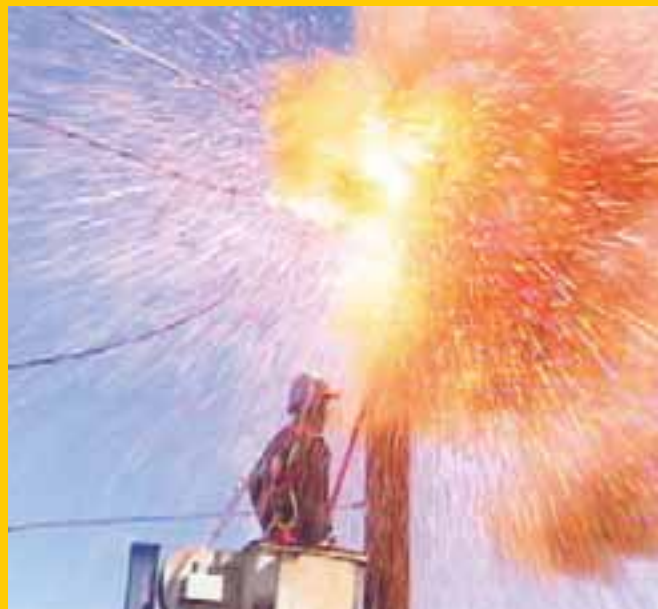
Con Edison Live Overhead Arc Flash Testing Manikin in a Bucket
