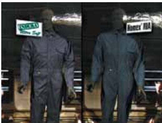
INDURA® Ultra Soft® and Nomex® IIIA garments before 3 second flash fire exposure.
