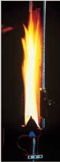
Vertical flame test on non-flame resistant fabric
