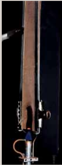
Vertical flame test on UltraSoft® fabric
